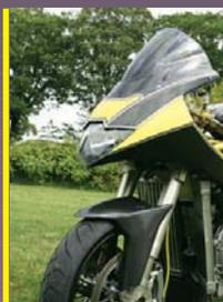
The GP Race suspension and the light-weighted brakes and carbon rims take care of an optimal road-holding. With diesel as fuel and the direct injection the motorcycle rides economically without giving in on power, speed and acceleration.
